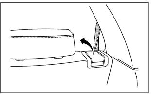
2. Lift the lever located on the top of the seatback to release the seatback and fold the seatback forward.
